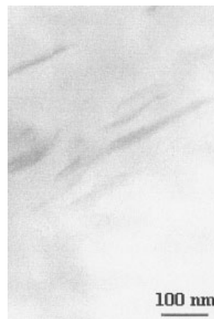
Figure 3 TEM image of PE-clay nanocomposite for containing 5wt% of TMD.
